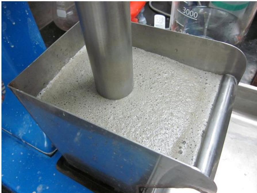
**Figure 1: Optimisation flotation test work.**
